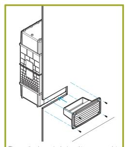
The weather louvre is designed to accommodate a variety of external wall thicknesses.
