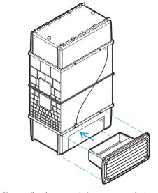
The weather louvre and storm cup are designed to slot into the air intake of the Silenceair 140mm unit.
