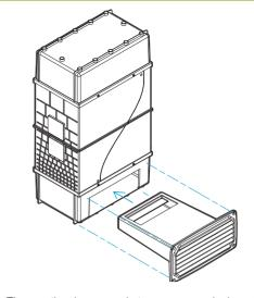
The weather louvre and storm cup are designed to slot into the air intake of the Silenceair 140mm unit.
