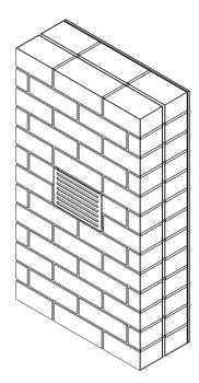
The Silenceair unit is completely hidden in the wall, only the period exterior grille is visible. 6
