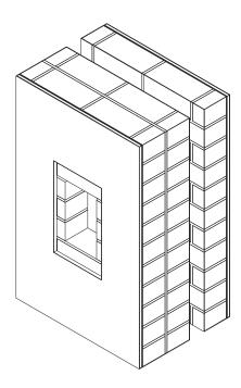
Chip away about 50mm of render on all sides of the interior opening to allow the fixing of the lathe plate (see image 5).
