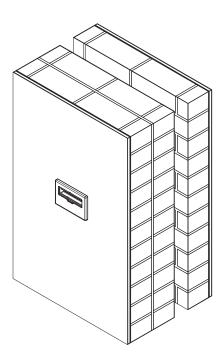
From the inside, the Silenceair module is completely hidden in the wall, only the adjustable face plate is visible.
