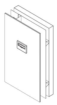
• From the inside, the Silenceair module is completely hidden in the wall cavity.
