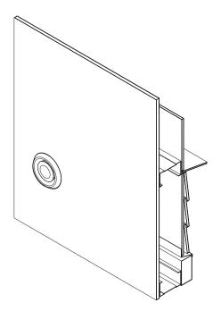
• From the inside, the Silenceair module is completely hidden in the wall cavity.
